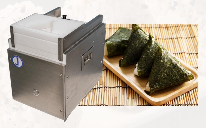
This Onigiri machine designed to make a triangular shaped rice balls filled with various ingredients, such as pickled plum, salmon, tuna, or vegetables, and wrapped in seaweed (nori).
