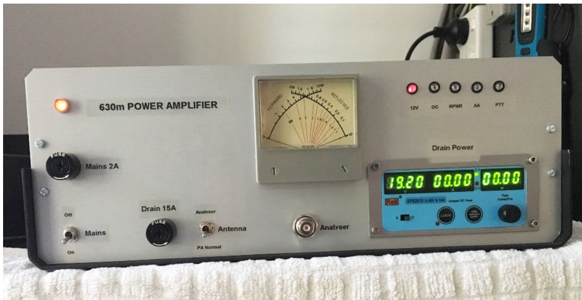
Figure 2. Front panel of VK6HP power amplifier. Note the switch to control the coaxial relay which routes the antenna to the antenna analyser BNC connector. Labels are printed using the LetraTag system and clear adhesive tape.
