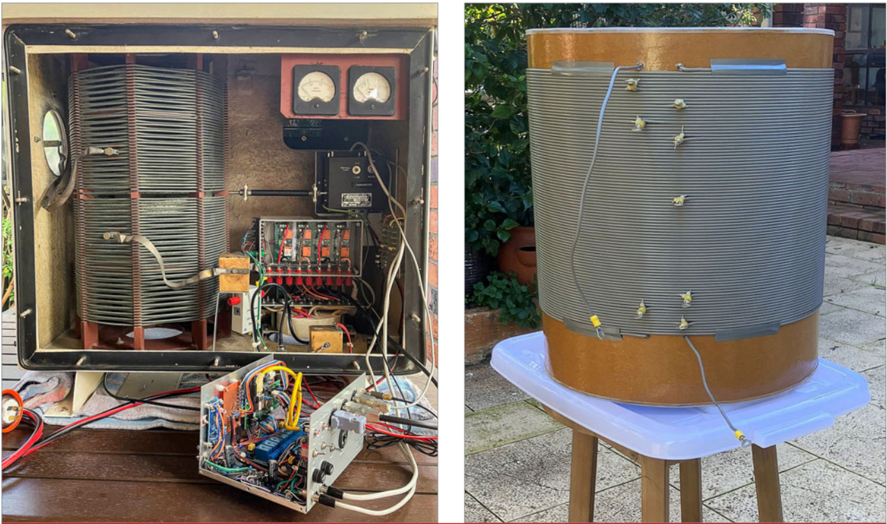
Figure 3(a). Department of Civil Aviation CU8A “aerial coupler” (modified for VK6MJM use) with the front access panel removed and the digital controller attached externally for bench testing. The impedance relay switching module (cover removed) is mounted above the original potted autotransformer assembly, while the RF current sensor monitors the current flowing to the variometer. The original “line” and “aerial” RF current analogue meters are still functional. (b) External 136 kHz loading coil (2.6 mH maximum).
