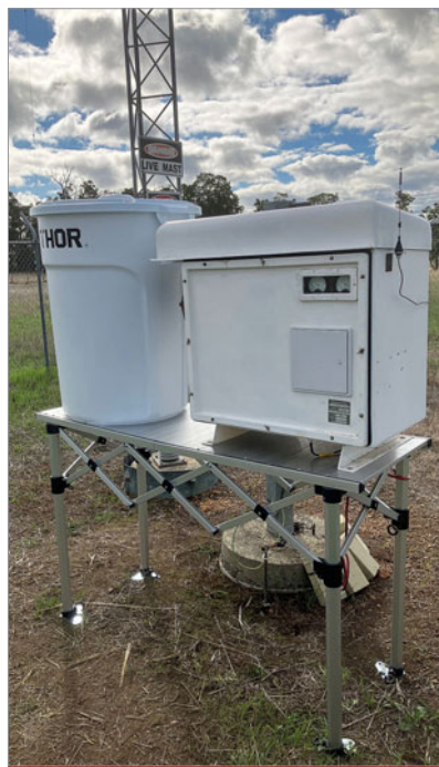
Figure 6. The Mark 2 coupler being tested in position near the base of the VK6MJM mast. The external 136 kHz loading inductor sits atop a low-density polyethylene (LDPE) box in a ventilated LDPE waste bin (206 l, Thor brand). The loss tangent of LDPE is low ( < 0.001 ) at LF and MF, but the coil should be as far as possible from the ground and ferrous structures.
