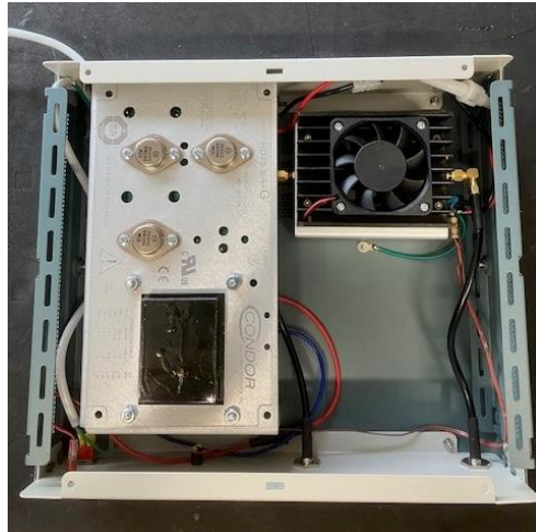
Fig. 5. (Left) Assembled bench power amplifier using a spare Schroff instrument enclosure. (Right) Internal view of the enclosure showing the 48 VDC 150 W linear power supply and PA. The power supply is secured via rear studs and the PA is mounted using strong Velcro.
