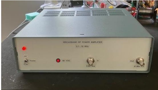
Fig. 5. (Left) Assembled bench power amplifier using a spare Schroff instrument enclosure. (Right) Internal view of the enclosure showing the 48 VDC 150 W linear power supply and PA. The power supply is secured via rear studs and the PA is mounted using strong Velcro.
