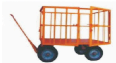
Door Type Platform Truck Capacity : 500kgs to 2000kgs Size : Diferent Length X Width X Height
