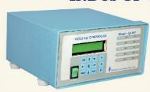
INDUS CP controller model CP402 controls the Carbon Potential (CP) inside a heat treatment furnace following one of the 50 set programs selected by the user. It takes its inputs from the Oxygen Sensor (Zirconia oxygen probe or Lambda sensor), thermocouple output representative of the process and uses these data to compute CP. These parameters as well as the measured temperature are used for control.
