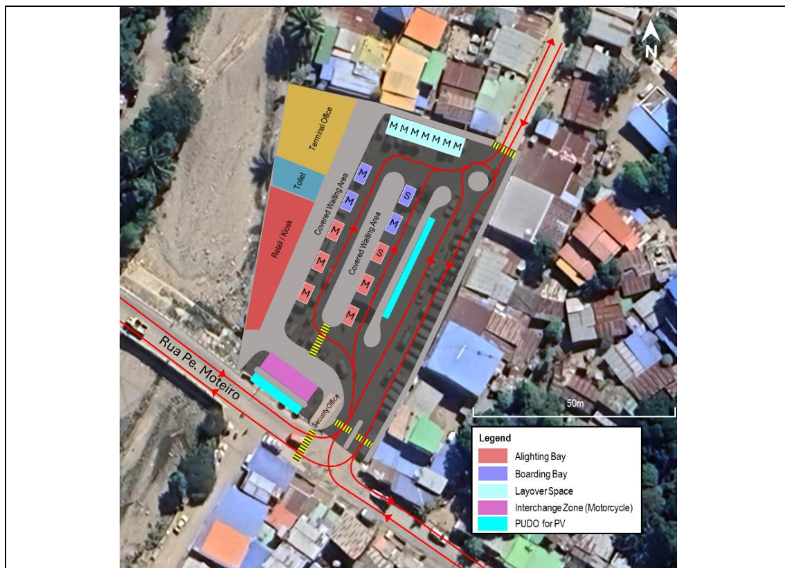
Figure 3-8: Preliminary Layout/Design for Becora Terminal
