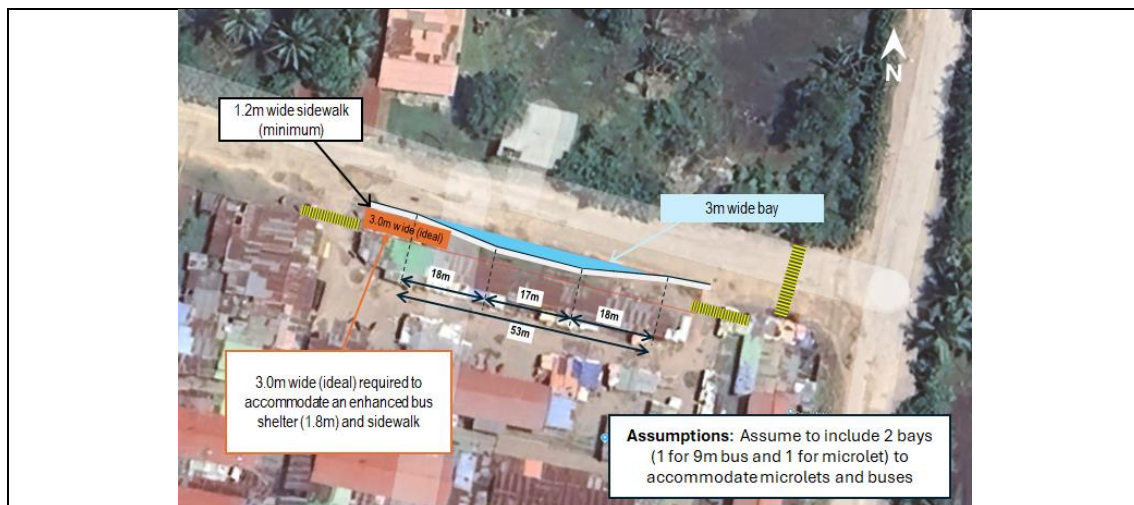
Figure 3-37: Preliminary Layout/Design for Lospalos Bemoris
