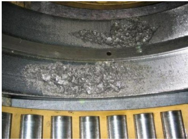
Image 52: Damaged outer ring of the large bearing
