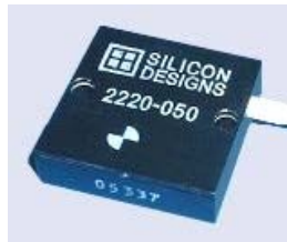
Image 21: An example of MEMS accelerometer
