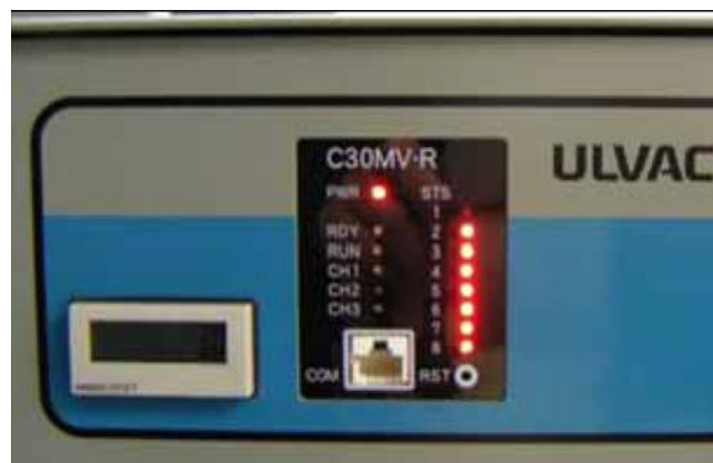
Figure 7-3: Reverse Phase or Phase Loss
