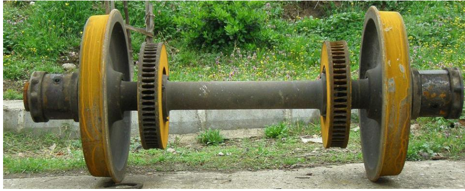
Figure 15.2 TVS 2000 type wagon wheel set
