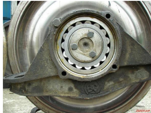
Figure 15.3 Axle bearing and axle box (cover removed)
