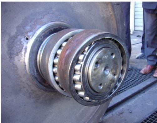
Figure 15.3 Axle bearing and axle box (cover removed)
