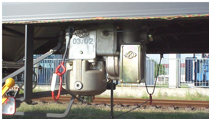
Figure 19.6 Triblivalve and mounted load relay valve
