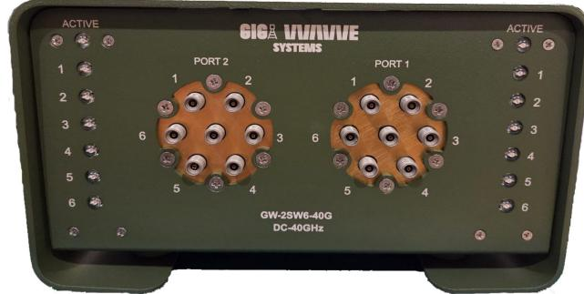
The Gigawave GW-2SW6-40G features two independently controlled electro-mechanical single-pole Six-throw (SP6T) switches, operating from DC to 40 GHz with high isolation and low insertion loss. These absorptive switches are designed with a failsafe, break-before-make configuration and offer a typical lifespan of 2 million switching cycles when operated within the specified conditions.
