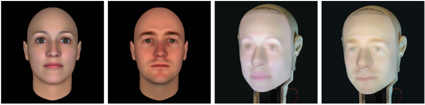
Fig. 1. From left to right: 2D image export from FaceGen showing the female and male face, 3D projection of the FaceGen female and male texture to the Furhat mask.
