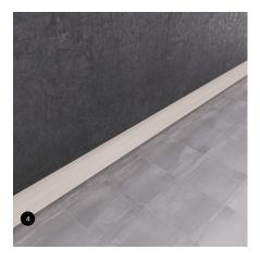
After the installation of the base flooring and ensuring it is level, proceed with installing the profile using tile adhesive. To enhance adhesion, consider adding 10% of 'Addibond' to strengthen the attachment to concrete.
