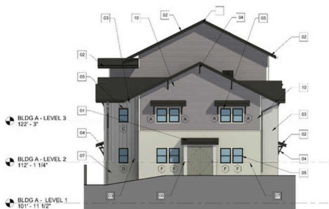
3 BUILDING A WEST ELEVATION SCALE: 1/8" = 1'-0"
