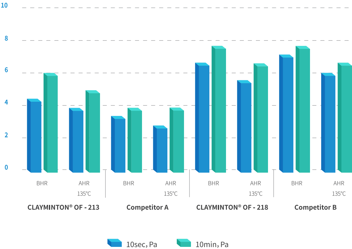
GEL STRENGTH COMPARISON,IN DIESEL OIL DRILLING MUDS (O/W=70:30)
