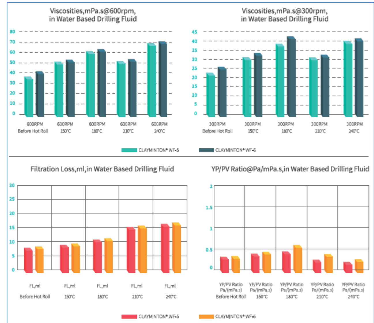
Rheological and filtration properties of water-based drilling fluids with WF-5 and WF-6.
