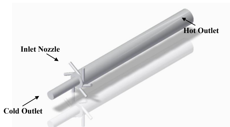
Figure 2. 3-D model of a vortex tube with inlet and exit conditions
