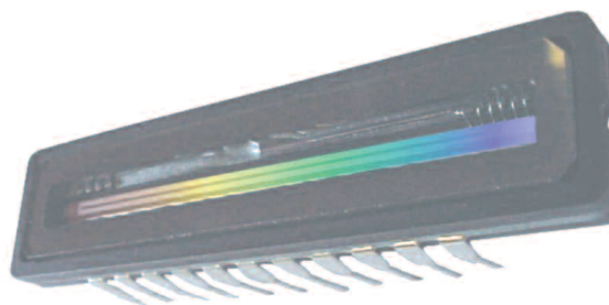
Figure 2 High-sensitivity, low-noise, 3648-pixel linear CCD array used in the 400 Series spectrophotometers (S.I. Photonics, Tucson, AZ).
