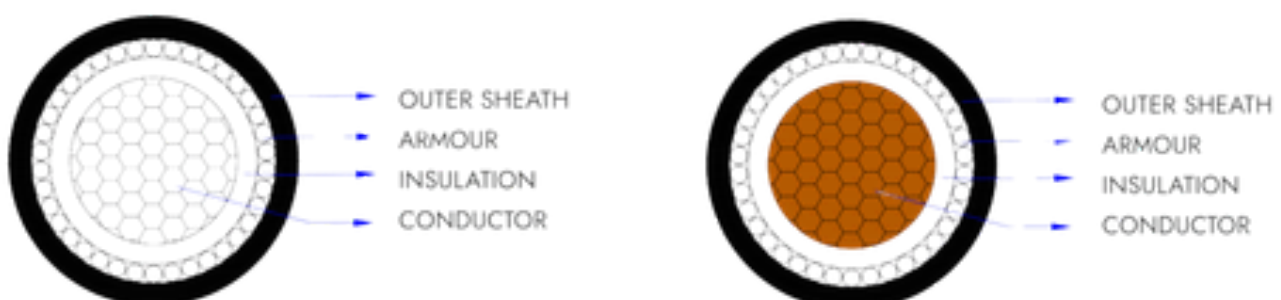
1 Core Round Wire Armoured Cable – A2XW 3 Y (ALUMINIUM) / 2XW 3 Y (COPPER)
