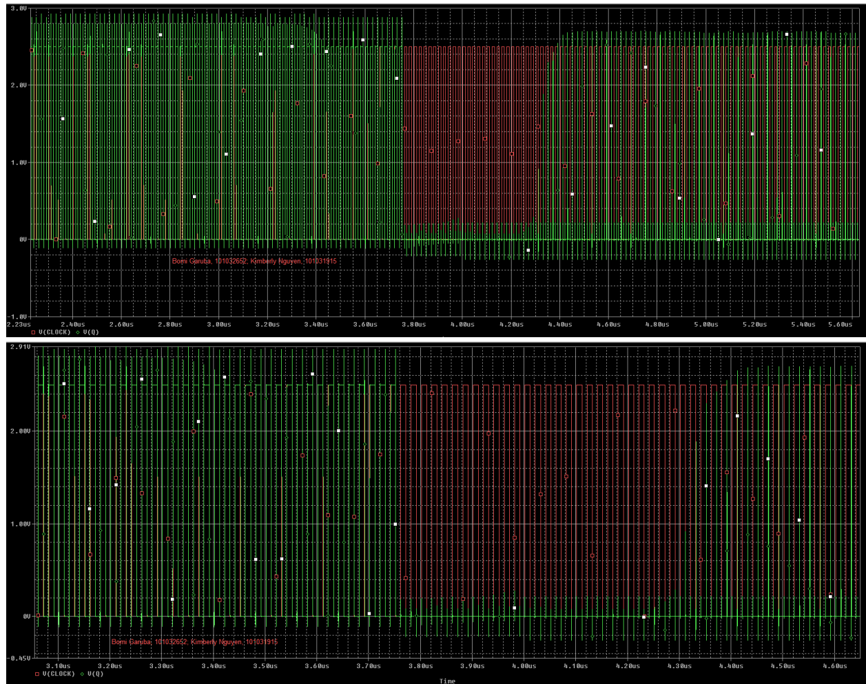
Fig 8. Waveform showing transparent latching
