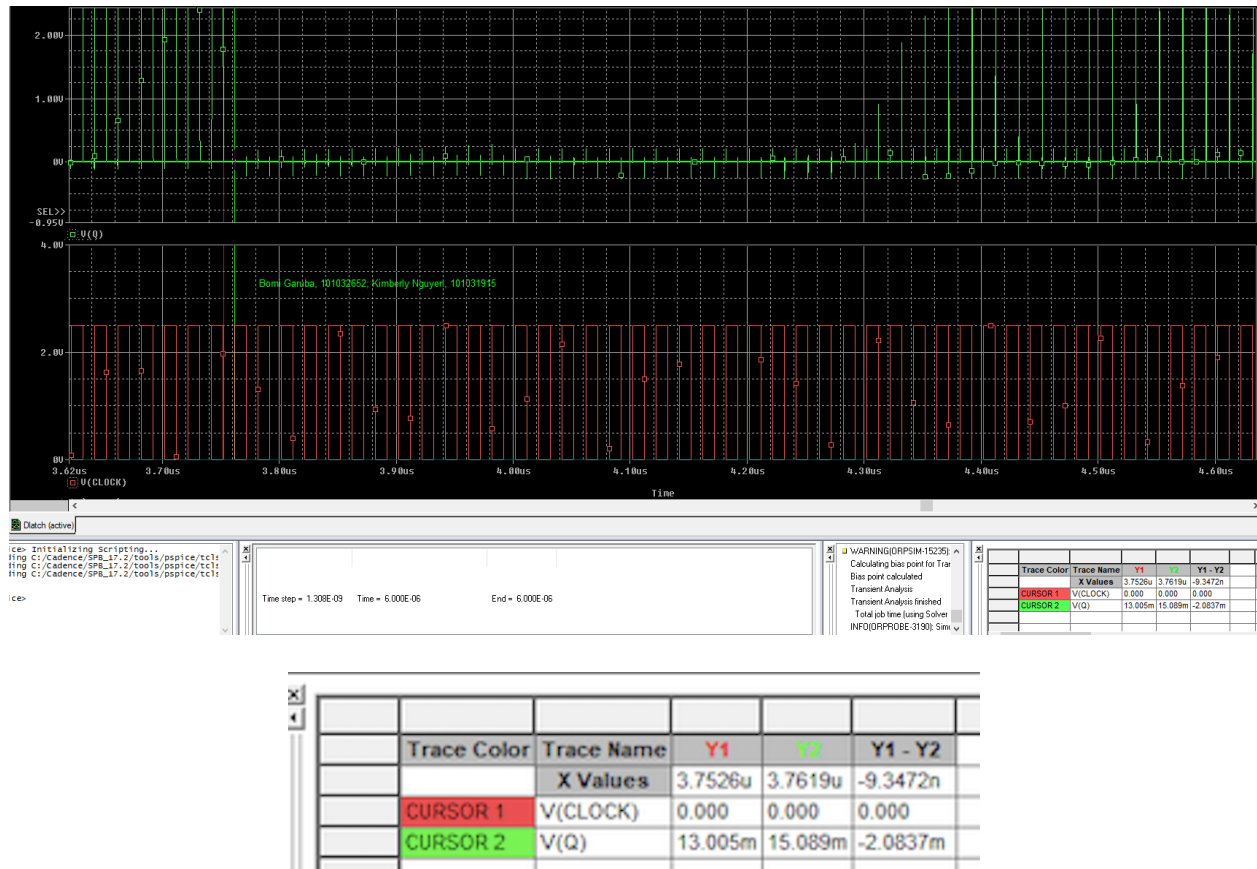
Fig 4. Measuring setup time for Latch circuit
