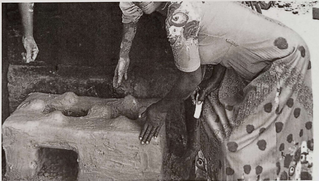
A two-hole family energy saving stove. Constructed using local materials and easy to repair
