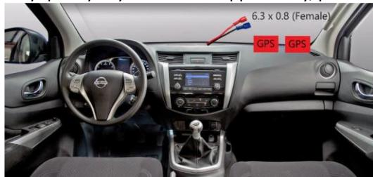
The position of the connectors must be in the car's front panel area
