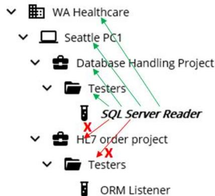
Figure 208.Accessible and Inaccessible References
