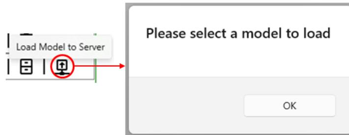
Figure 49. Load Model requires model selection
