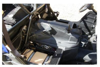
2. Unfold Dust Guard, place over seating area & insert seat belt latches through holes.
