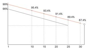
AIRMAC Solar linear power output guarantee Standard linear power output guarantee
