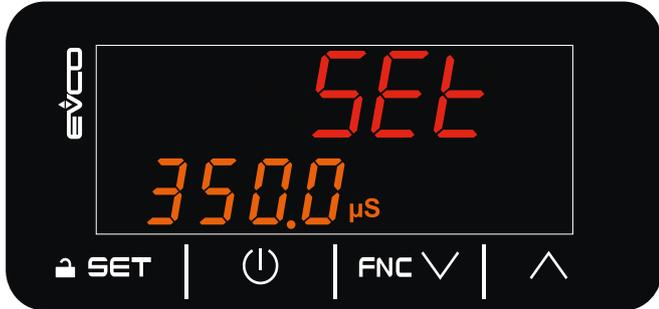
Fig. 4. First start-up - Setting the electrical conductivity
