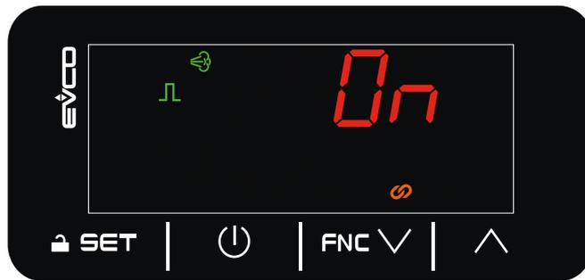
Fig. 6. Home screen with ON/OFF regulation from digital input (CFG = 0-1)
