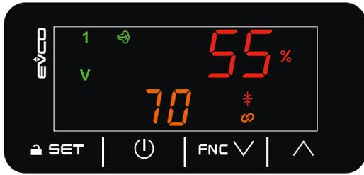
Fig. 8. Home screen with humidity sensor alone
