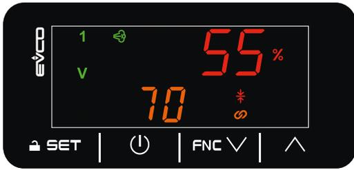
Fig. 36. Home screen with humidity sensor alone
