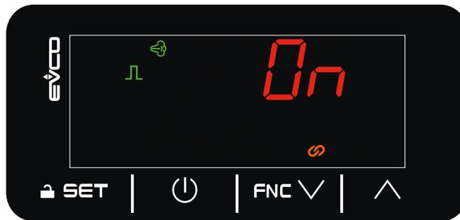
Fig. 34. Home screen with ON/OFF regulation from digital input (CFG = 0-1)
