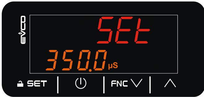
Fig. 32. First start-up - Setting the electrical conductivity
