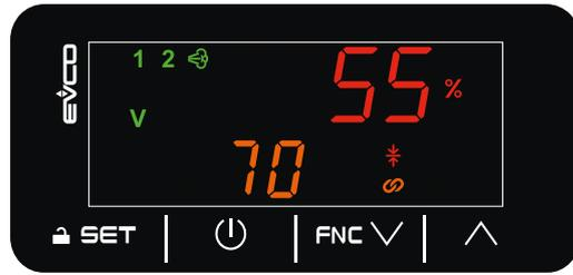
Fig. 37. Home screen with humidity sensor and limit sensor
