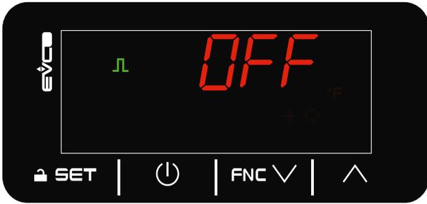
Fig. 27. ON/OFF operation - ID1 and ID2 open
