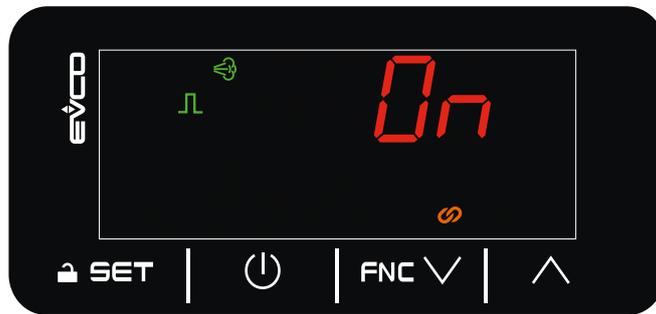
Fig. 56. Home screen with ON/OFF regulation from digital input (CFG = 0-1)
