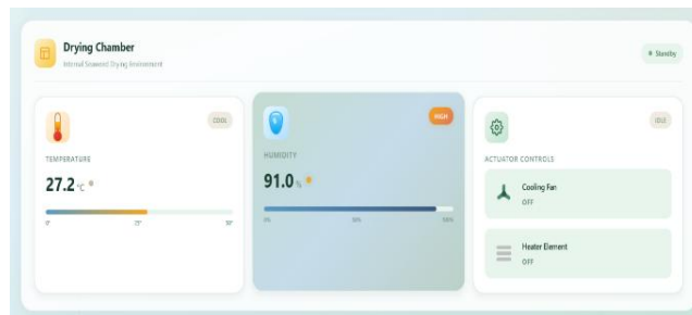
Figure 10. Real-Time IoT Dashboard Showing Drying Chamber Temperature, Humidity, and Actuator Status
