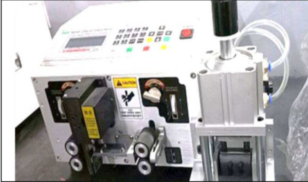
Fully automatic Wire cutting, stripping
