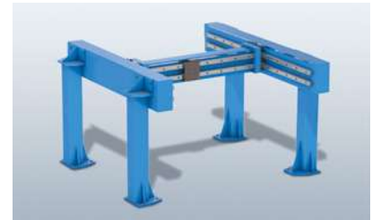
Synchronization of the feed motors for gantry drives with a separate measuring system
