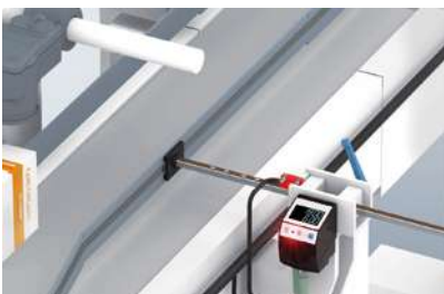
Monitored lateral guidance in packaging machines
