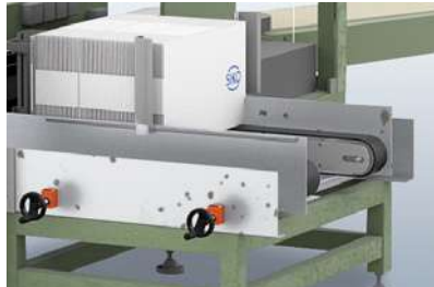
Reproducible adjustment of cardboard box erecting machines
