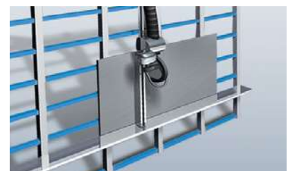
Direct display of the measured values on a vertical panel saw
