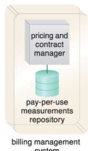
Figure 9.9 A billing management system comprised of a pricing and contract manager and a pay-per-use measurements repository.
