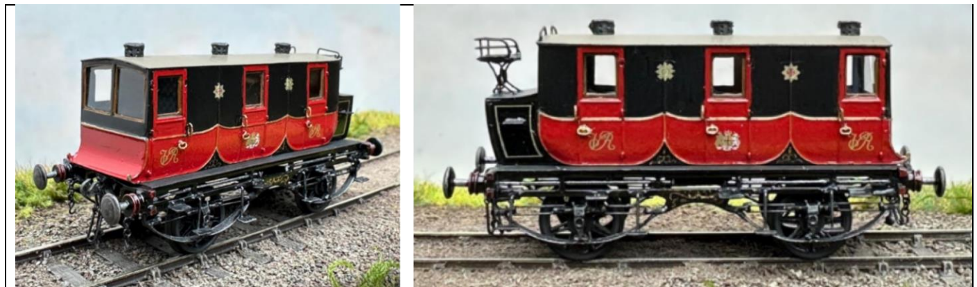
Chris' model of the London & Birmingham Mail fitted up for Queen Adelaide in 1839. The bow springs were much liked by early commentators as they gave a sense 'of the finest texture and admirable elasticity'. Ref: model and photo Chris Cox
