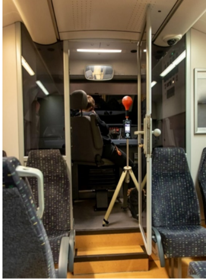
Measurement of the driver cab and sitting area using the portable EMF meter
