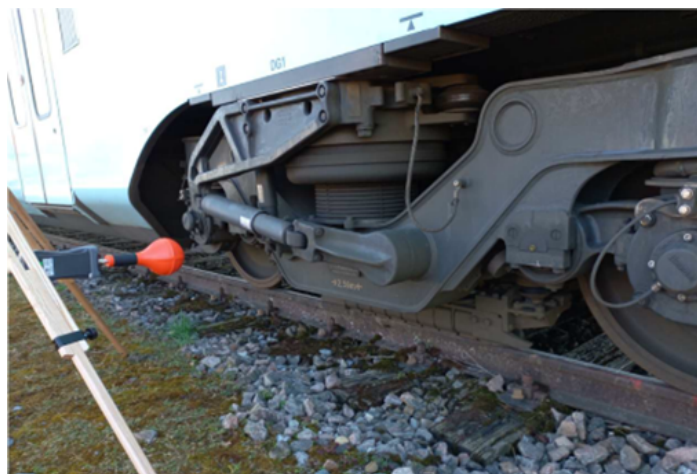
Measurement of the bogie and mag-braking system of the rolling stock
