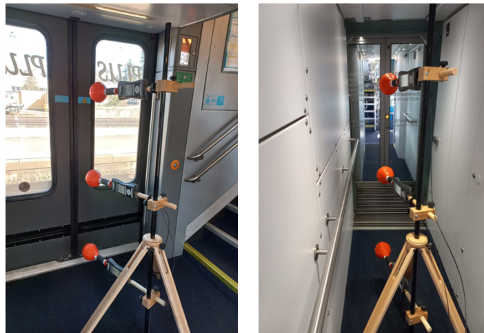
Simultaneous measurement heights at 0.3 m (public area), 0.9 m and 1.5 m (public and worker areas)
