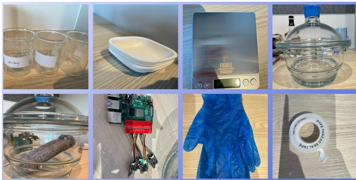
Figure 3. Materials and hardware used for odour data acquisition, including glass beakers, weighing dishes, precision scale, sealed glass chamber, Raspberry Pi with sensor boards, gloves, and PTFE tape. (Photographs by Yiyi Zhang, 2025.)
