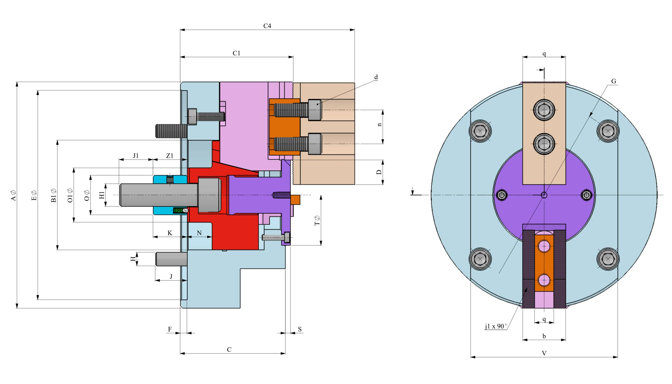
Two jaw chucks are pre dominantly used when machining irregular shaped components and are therefore mainly used with contour jaws.
