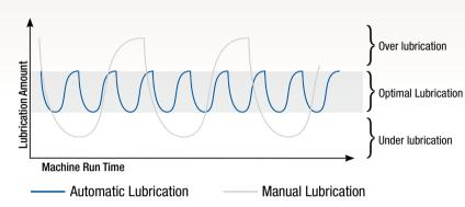
Excess heat build-up, faster component wear and wasted lubricant adds up to unnecessary labour costs, material costs, and higher energy consumption. With Graco automatic lubrication equipment you'll be sure to get the most from your equipment and more productivity per machine operator.
