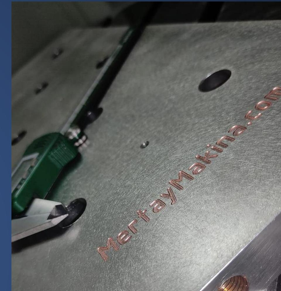
*“One of the custom cooling plates designed, thermally analyzed, and manufactured in-house for CERN’s Large Hadron Collider (LHC) infrastructure.”*
