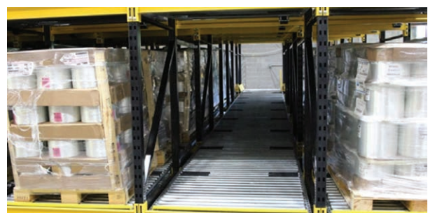
Pallet Flow Racking with solid rollers.
