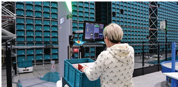
A picker picks from a tote bin brought to a pick station by an AMR and tote AS/RS solution.
