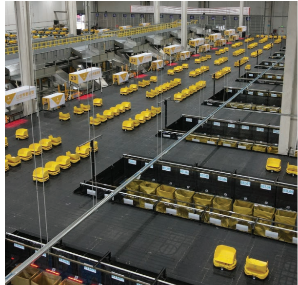
Sorting and picking operation powered by AMR technology.
