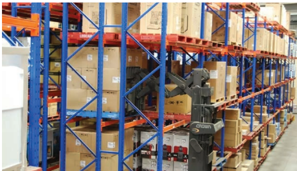
Example of double deep rack with special mast lift truck.
