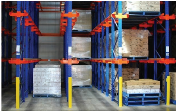
Example of a LIFO drive-in racking system.
