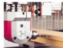
Tilted side boring
