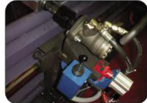
Optional: Hydraulic Wrench Tightener and Auto. Fix - in system.
