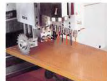
Pneumatic line boring
