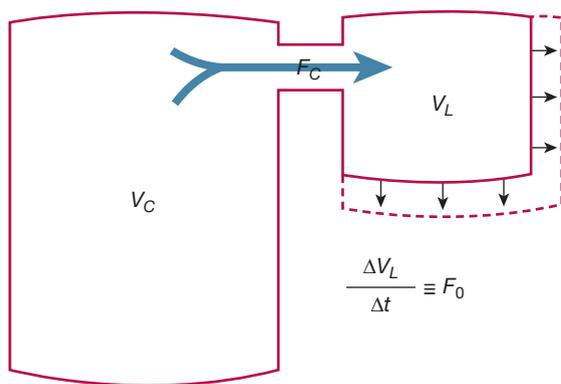
Figure 3 – Diagram showing the physical basis of the MiniBox method. A rigid container of volume  $V_C$  is connected to a container of volume  $V_L$  which expands at the rate  $F_0$ . Here  $V_L$  mimics the lungs and  $V_C$  mimics the volume of the MiniBox device. The rarefaction of gas in the expanding system induces a flow of gas  $F_C$  from the rigid container to the expanding container.
