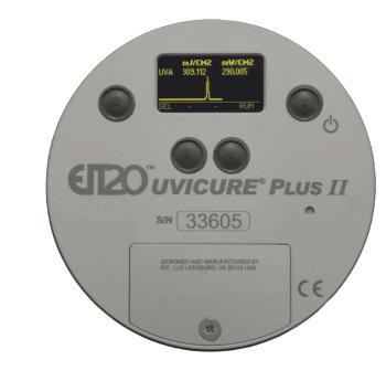
The UviCure Plus II is a single-band UV radiometer developed by EIT 2.0 LLC, designed for broadband UV curing systems. It is widely used in industrial applications for monitoring, documenting, maintaining, and troubleshooting UV curing conditions.
