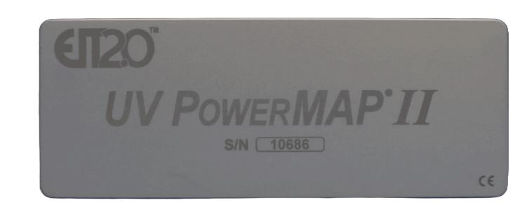
The PowerMAP II is a profiling UV radiometer designed by EIT 2.0 LLC for measuring broadband UV **sources** across four spectral regions (UVA, UVB, UVC, UVV). It captures:
