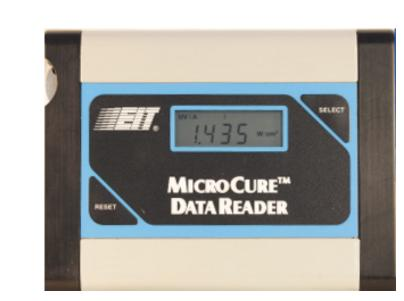
The MicroCure® is a compact, single-band UV radiometer developed by EIT 2.0 LLC, designed for small or hard-to-reach UV curing environments. It measures both energy density (J/cm²) and peak irradiance (W/cm²), making it ideal for quality control in tight or high-temperature spaces. MicroCure® UV radiometer. It enables users to toggle between irradiance (W/cm²) and energy density
