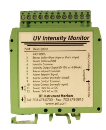
The EIT 2.0 On-Line Monitoring System delivers real-time UV intensity feedback using durable Compact Sensors and DIN Rail units. Ideal for LED or broadband sources, it ensures process control in tight, fast, or hard-to-access environments—helping you maintain quality, reduce scrap, and catch issues before they impact production.
