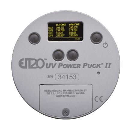
The UV Power Puck II Profiler is a four-band profiling UV radiometer developed by EIT 2.0 LLC. It combines an easy-to-use display interface with advanced data profiling capability for in-depth UV system diagnostics, process validation, and quality control.
