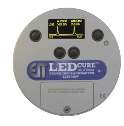
The LEDCure® is a compact, battery-powered UV radiometer developed by EIT 2.0 LLC. It is designed specifically for industrial UV LED curing systems, providing accurate and repeatable irradiance (W/cm²) and energy density (J/cm²) measurements, as well as a graphical irradiance profile. Built for ease of use and field reliability, it features EIT's patented Total Measured Optical Response (TMOR) for precise absolute energy measurement.
