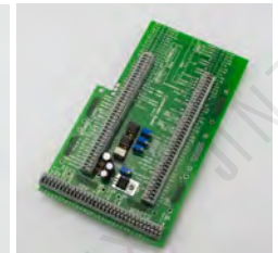
Main Board For Laser Cutting M/C
