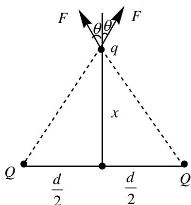
$$F_{net} = 2F \cos \theta \quad F_{net} = 2 \frac{KQq}{x^2 + \frac{d^2}{4}} \cdot \frac{x}{\left(x^2 + \frac{d^2}{4}\right)^{1/2}} \quad F_{net} = \frac{2KQqx}{\left(x^2 + \frac{d^2}{4}\right)^{3/2}}$$
